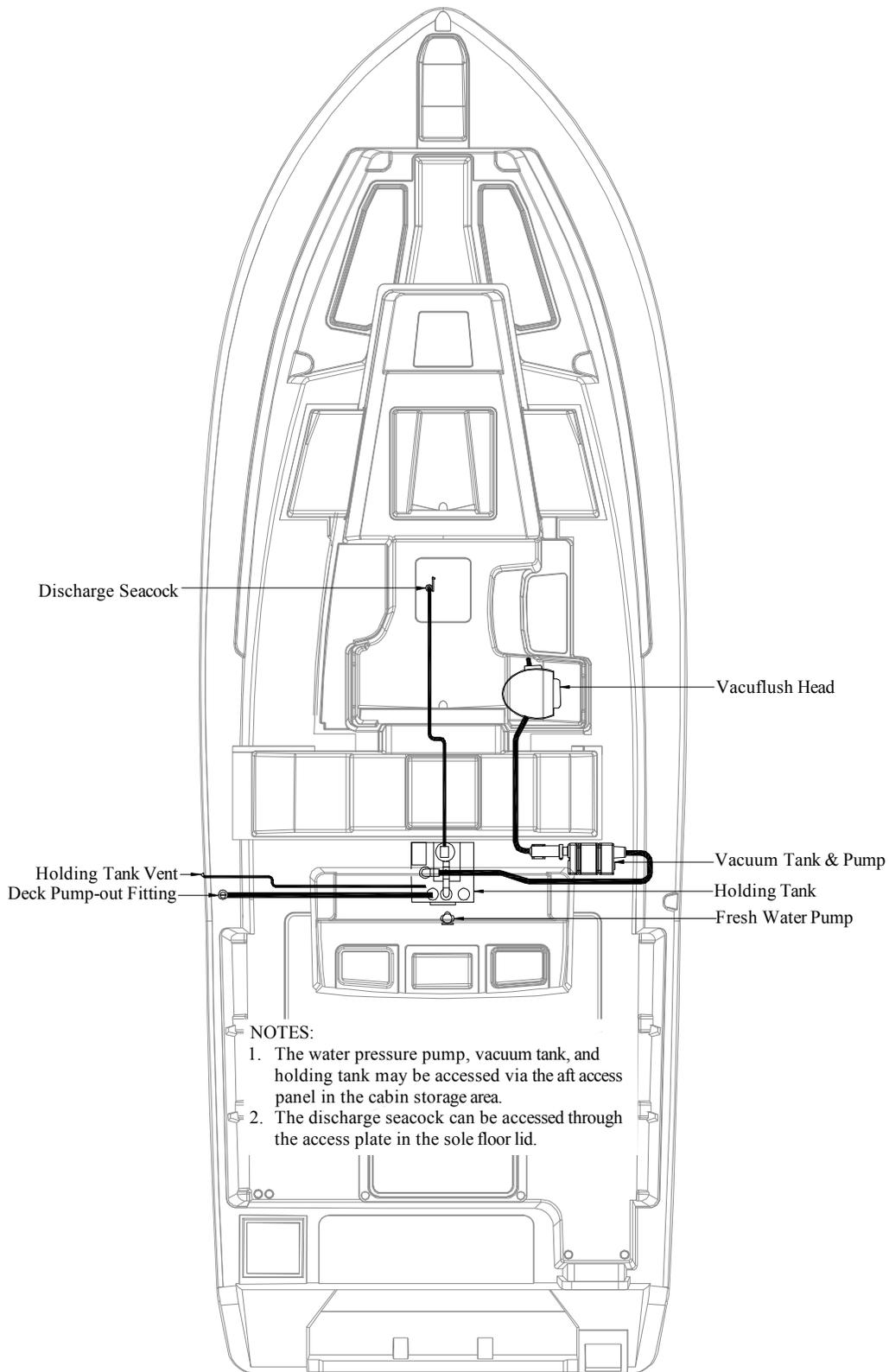
*Pressurized Freshwater System Layout*
