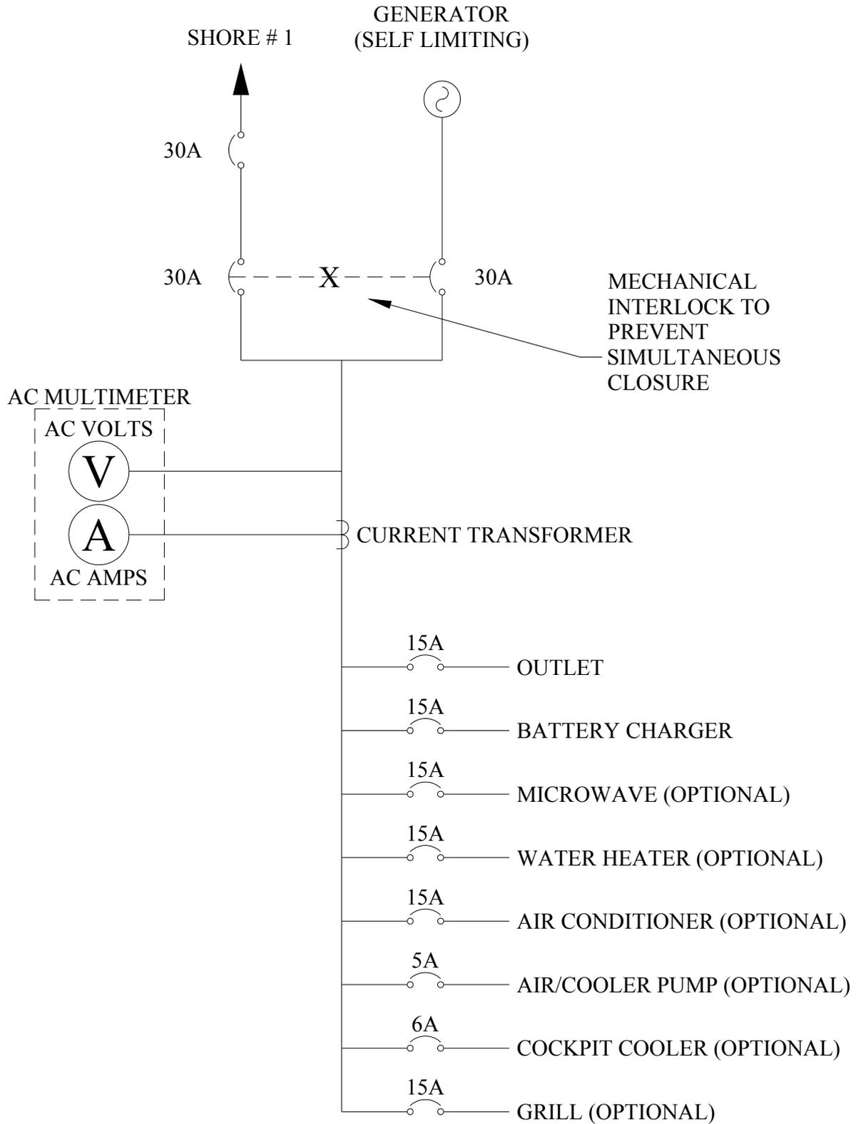
*120V Cockpit Cooler One-line Diagram*
